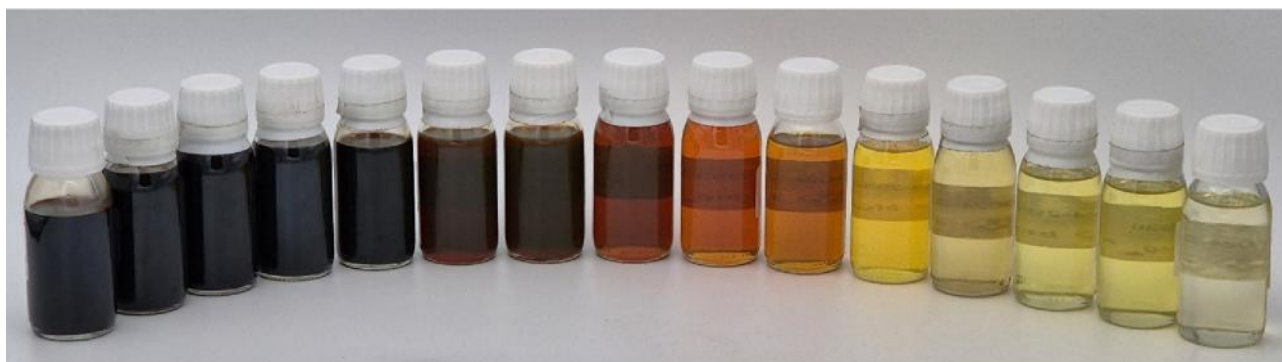
Figure 5. Different qualities of HPO produced; hydrotreatment severity increases from left to right.
